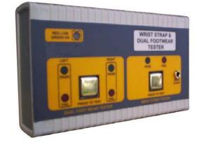
**Operation of Wrist Strap:** Connect the wrist strap cord to the instrument with the strap on the wrist; press gently on the metal sensor of the wrist strap tester. The instrument comes on automatically when this is done. The operator can check whether the resistance of the wrist strap falls within the acceptable range (0.75 to 10 Meg ohms), This is indicated by green (pass) LED lighting up.
