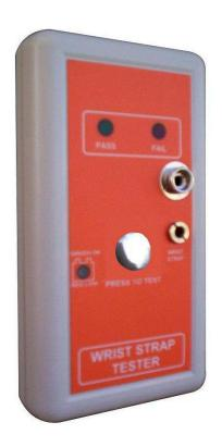
It clearly indicates whether or not the resistance of the wrist strap system including the wearer is at least 0.75 Meg ohms and not more than 10 Meg ohms respectively.
